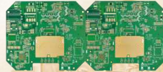
Layers Count: 6L (ENIG) Min drill hole diameter: 0.25mm Line Width/Space: 0.152/0.102mm Application: Network Communication
