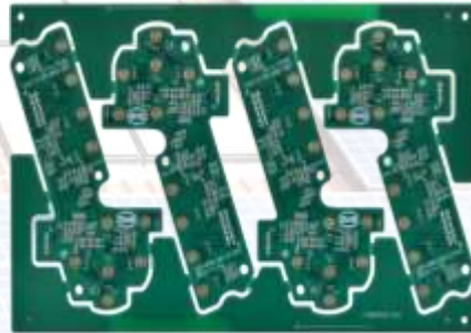
Layers Count: 2L(ENIG) Min drill hole diameter: 0.40mm Line Width/Space: 4/4mil Application: Automotive (Dashboard)
