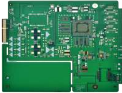
Layers Count: 6L (OSP+ENIG) Min drill hole diameter: 0.35mm Line Width/Space: 3/3mil Application: TV Mainboard
