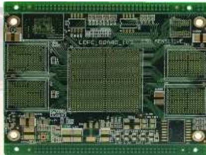
Layers Count: 10L (OSP) Min drill hole diameter: 0.25mm Line Width/Space: 3/3mil Application: Server
