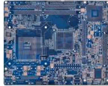
Layers Count: 4L (OSP) Min drill hole diameter: 0.20mm Line Width/Space: 3.9mil Application: Consumer electronic
