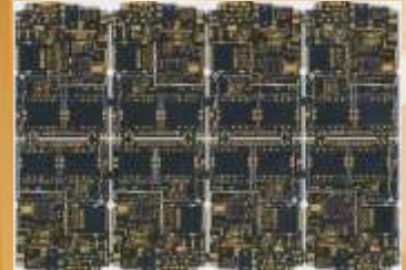
Layers Count: 4L(OSP+ENIG) Min drill hole diameter: 0.25mm Line Width/Space: 4/4mil Application: Feature Phone
