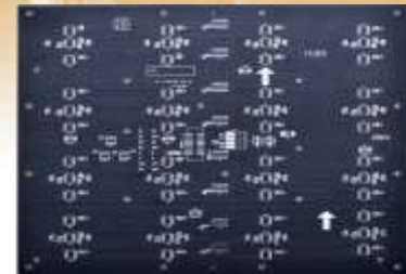
Layers Count: 4L(HASL LF) Min drill hole diameter: 0.30mm Line Width/Space: 5/5 mil Application: LED Display
